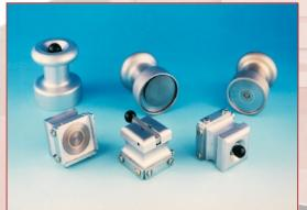
A small vice for circular samples  $\phi$  32 - 45 mm, height 4 - 10 mm.
