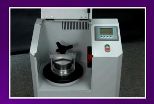
The instrument enables a very quick milling of small quantities of various kinds of materials and their simultaneous homogenization.
