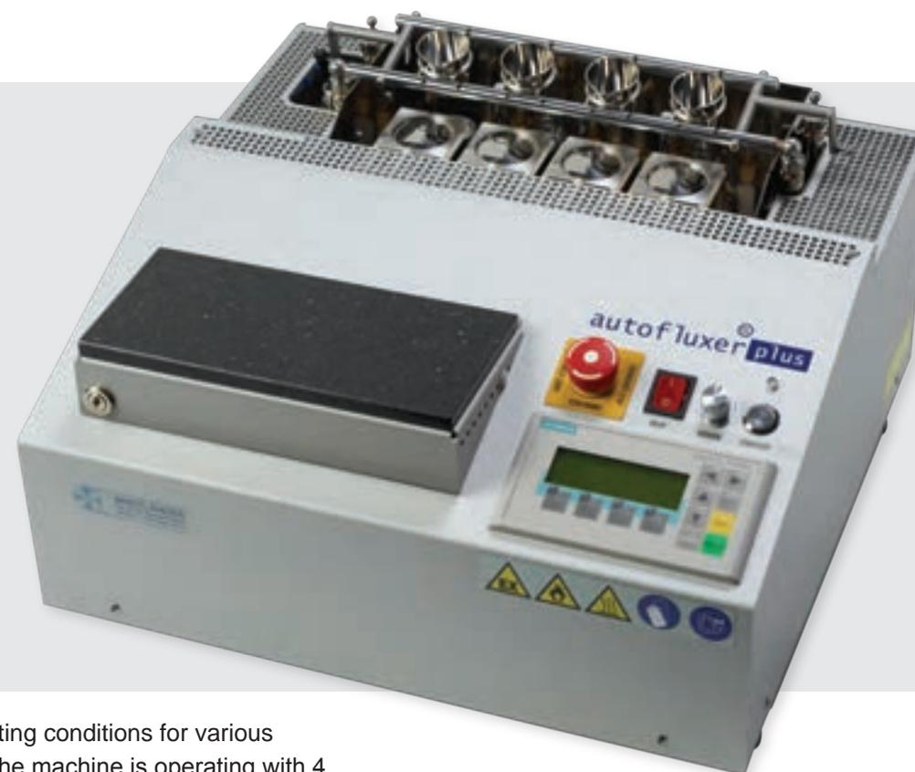
This machine is especially designed for routine analysis, when reproducible melting conditions for various materials with specific fusion parameters are required, independent of whether the machine is operating with 4 stations or in between for some single sample on 1 or 2 stations only.
