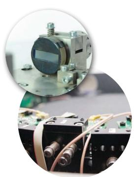
The GDA 550 HR is an exceptionally sensitive high-performance spectrometer to determine the chemical composition of surfaces and coatings. With up to 79 analytical element channels, using photomultiplier tubes, the GDA 550 HR glow discharge spectrometer is the perfect tool for applications requiring flexibility, high resolution, and analytical precision.
