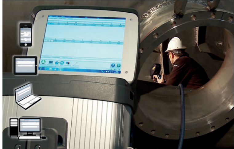
WebApp - Typical use when direct view to measurement screen is not possible
